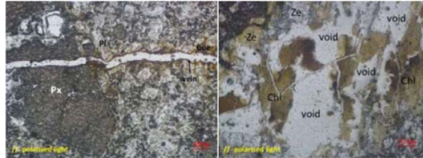
Figure 5. Photomicrographs showing secondary mineral types, vein and fractures on ST-250 and ST-260 Basalt samples
